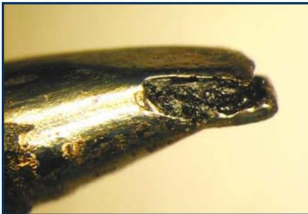
The picture on the left shows a tip destroyed by tin erosion when using lead-free solders. In this case the tip life was only three weeks. Traditionally the user had been used to a tip life averaging 3 months with leaded 63/37.
